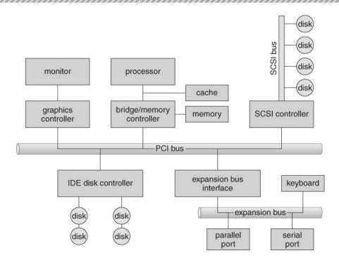
Fig: A Typical PCI Bus Structure
