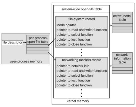
Figure 13.12 - UNIX I/O kernel structure.
