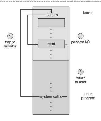
Fig: Use of a system call to perform I/O.
