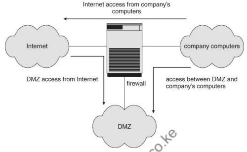
Figure 15.10 - Domain separation via firewall.
