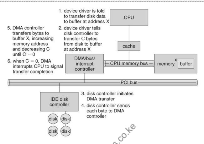
Fig: Steps in a DMA Transfer
