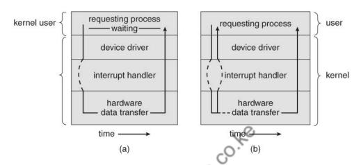
Fig: Two I/O methods: (a) synchronous and (b) asynchronous.
